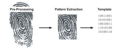
The verification procedure (figure 4) begins with the pre-processing of the incoming fingerprint image. The registered small images from the template are then compared with the fingerprint image to determine to what degree the template matches the image. A threshold describing the smallest allowable deviation is then used to decide if the finger matches the stored template.
